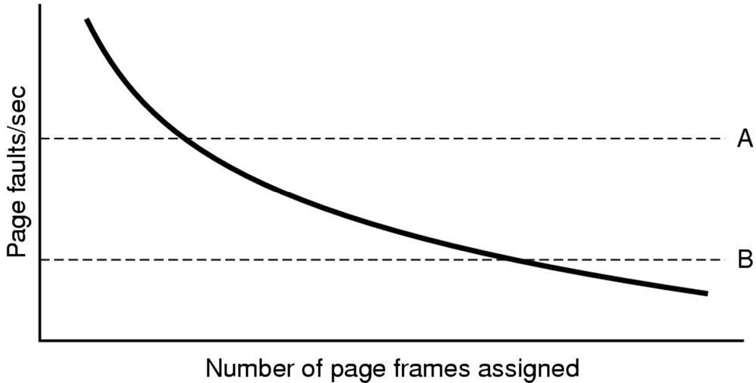
Page fault rate as a function of # of page frames assigned
